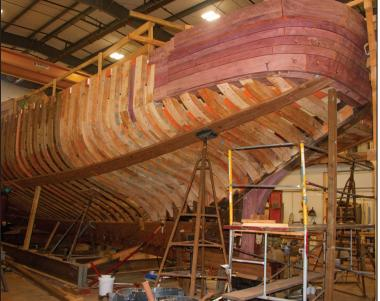
The graceful lines of the Western Flyer are on display in this view of the port flank. Ribs have been bent into place, ready for planking to be laid up, sealing the new hull of the 1937 purse seiner built in Tacoma for the Monterey, California, sardine fleet.
