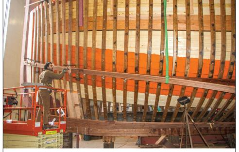
Shipwright Ryan Bard clamps a first plank in place where it cools into the complex shape of the hull from stem to stern.
